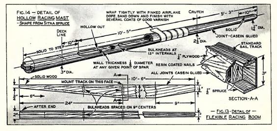
The racing spars are built as shown above. The mast is stepped in the usual manner. In hollowing out the mast carefully follow directions in the text. Note that bulkheads are spaced on 9" centers in the flexible racing boom above.
