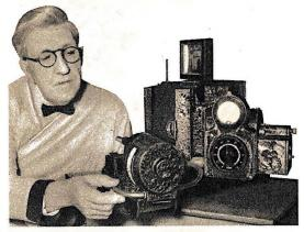
W. F. Alder, California research scientist, developed the "polyscope", shown above, in his garage-laboratory. With it three-dimensional movies are made and projected on screen.
