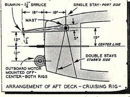
To give rudder and tiller free play the mizzen mast and outboard motor, if used, are placed off center as shown above. Shape of bumkin and rigging are also given in detail.
