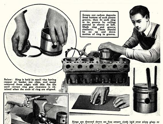
Rings are dressed down on fine emery cloth laid over plate glass or planed hardwood surface. Rings are slipped off pistons with hacksaw blade skids, replaced with skids in same manner, bottom ring first. Above: Using adjustable type piston ring compressor to put piston back.
