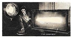
A light meter placed in the fog chamber measures variations in beam intensity as atmospheric conditions are changed.
