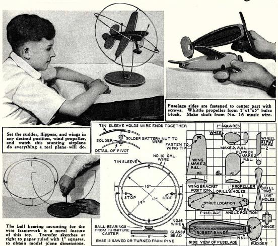
A RUBBER-BAND powered model airplane of any type, mounted in this tilting, whirling, rolling cradle, will provide hours of keen amusement, and at the same time show just how all the different maneuvers of an airplane are carried out. When the rudder, flippers, and wings are set for a particular stunt and the motor wound, the model will respond just as faithfully as would one of the Navy's stunting Hell Divers. End over end spins, Immelmann turns, tail spins are all possible with this little toy.
