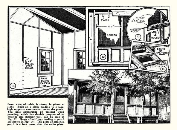
a two-inch seat on pier, then spike securely to sill. At intervals of 2', center to center, notch for butting in half-log studs. Join trimlog corners with a miter cut, as shown in Fig 2. Trim-logs should be large enough to extend above the sill. The joists of 2" by 6" material, spaced 18", center to center, are butted to the sills and rest on a central 6" by 6" beam. Spread rough boards over joists for temporary flooring.
