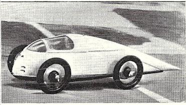
Victor Stafford, famous British racer, is seen at the controls of a new powerful midget car which will attempt to break existing international speed records. The car has its engine behind the driver who must be lowered into his car and the cowling placed over him. The auto resembles an airplane stripped of wings.
