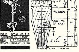
In either the ketch rigged cruiser or outboard cruiser dean eitner the ketch rigged cruiser or outboard cruiser designs, do not use a motor over five h.p. If you plan to use a motor as auxiliary power, the outboard motor mount above must be fitted to the transom and the transom reinforced with brackets. Fig. 11 shows shape of the bowsprit.
