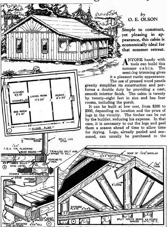
Fig. 1 shows floor plan of the cabin which can be changed to suit builder. The 2"x6" floor joists in Figs. 2 and 3 rest on a 6" square beam running down the center of the floor plan. It is advisable to use concrete piers under this beam also. The sunburst effect in Fig. 4 is an attractive feature, yet provides a sturdy support for the roof.
