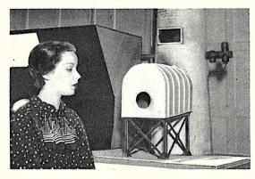
A model of a factory smoke-stack equipped with an electric eye is shown above. When the chimney smokes, a photo-electric cell quickly detects fuel waste and warns fireman.
