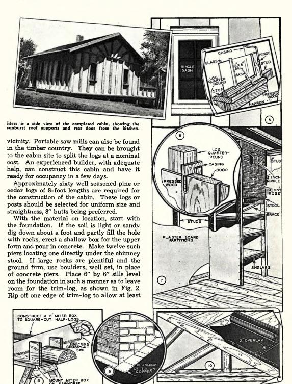
By building the miter box in Fig. 8 square cutting of logs will be simplified. The chimney rests on a stool five feet above the floor. Shelving, built into the stool, provides pantry space in the kitchen. Lay roofing as shown in Fig. 10.
