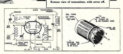
VOICE and music programs can be broadcast through your own radio receiver with this midget one-tube transmitter, the world's smallest radio station. Weighing less than two pounds complete with batteries when ready to go "on the air," the entire unit fits into a five-cent bread pan measuring less than 2"x4"x7" in size.
