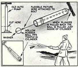
Hollow rubber ball, fastened to plunger of revamped tire pump, gives loud report when pump handle is depressed.
