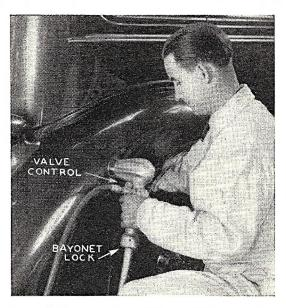
Pneumatic hammer, striking 4,000 powerful blows per minute, simplifies car body and fender straightening. Speed-regulated, equipped with eight changeable dies to fit contours of modern car, trigger-operated device is claimed to save hours of hand hammering. U-shaped metal yoke holds the die close to the hammer when used in straightening work.
