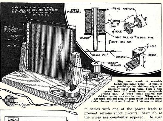
This diagram shows how to connect home-made circuit breaker to electric fly killer. Solenoid bracket touches plunger.
