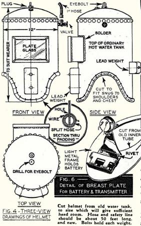
Radio earphones act as both transmitter and receiver in this simple communication system which permits diver to give instructions to man at surface. A 4½-volt C battery supplies the power—large battery may be used if more volume is desired. Two waterproof wites are run from helmet to surface.
