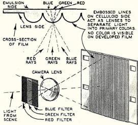
Lenses embossed in film provide color separation in Kodacolor process developed by Eastman Kodak to give color movies to amateur movie fans using 16 millimeter film. Both camera and projector must have the special threecolor filter, since finished Kodacolor film shows no color.
