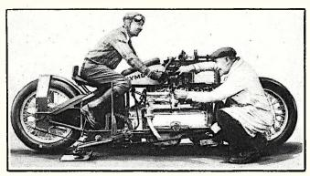
Fred Luther, Los Angeles racer, is shown seated on his specially built motorcycle with which he hopes to exceed 300 m.p.h. It is powered by a 6-cylinder auto engine. Note brake skid on ground in front of rear wheel.
