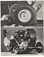
Two views of midget motor for use in operating wash-machines.
