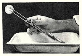
The danger of staining photo prints while passing through chemicals is eliminated with this set of wooden tongs.
