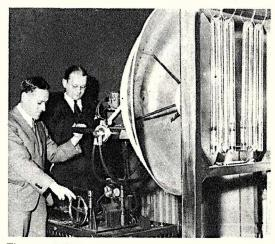
The new radio transmitter, shown above, operates on an ultra-short wave length of nine centimeters. Neon tubes are used to transfer voice signals to reflected wave beam.
