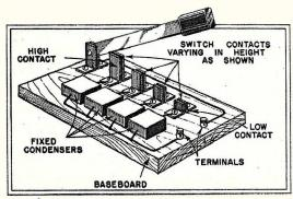
Total capacity between the terminals of this bank condenser is the sum of capacities which are switched into the circuit.
