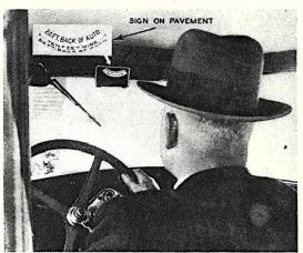
By means of new rear window reflector, image of a sign six by ten feet placed on the road two feet back of the car was reflected into rear view mirror over windshield to show parking advantages of new road-reflecting mirror for motorists.
