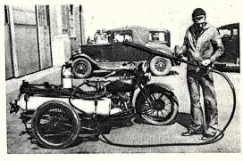
This unique fire extinguisher is used to smother plane flames at airports. Chemicals and hose are mounted on a three-wheeled motorcycle and rushed quickly to the scene.
