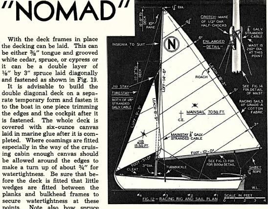
Here is Nomad rigged as a racing sloop. Mast and boom are hollow to reduce weight. Note breakwater ahead of cockpit to turn down waves washing over.
