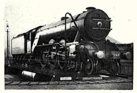
This English locomotive connects its vacuum brake pipe to a small motor to turn the table under its own power. Note vacuum tank under locomotive platform for power reserve.
