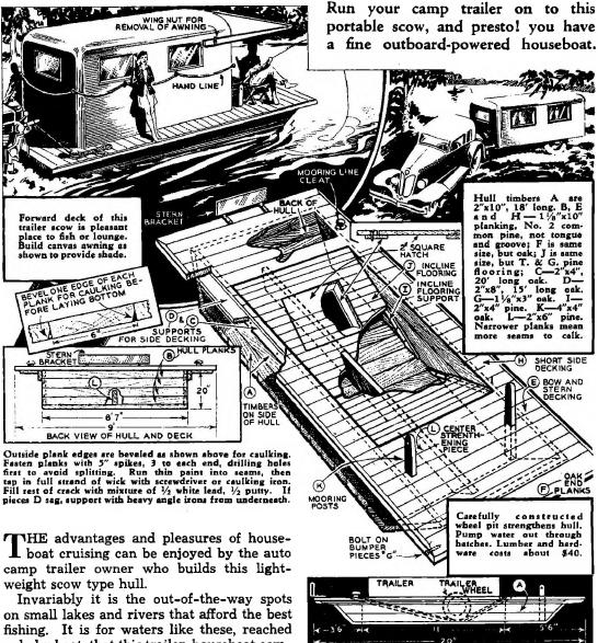
Side view of hull of scow showing how wheels fit into pit.
