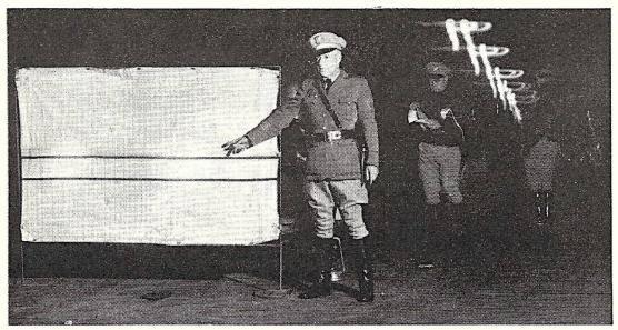
Captain Stevens of the California Highway Patrol points out a headlight test chart used in war on killer cars. Autos are stopped a definite distance ahead of chart; those whose headlight beams go above upper black line get tickets. More than 1,000 cars ordinarily pass through such a test trap in one shift. Unless defects in lights are corrected at once, fines are imposed.
