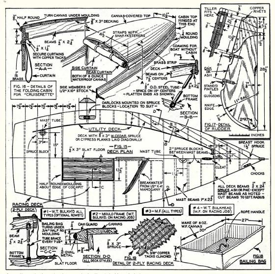
Carefully study these drawings as all details of decking, deck frames, coaming, cabin and flooring are covered thoroughly. The upper half of the deck plan (Fig. 15) is for the cruiser, while the lower half gives details of the racing sloop.
