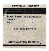
Above sketch shows cross-section of new 16 mm. color film. the three-color sensitive emulsions separated by gelatin layers. Or-dinary filming requires no filters.
