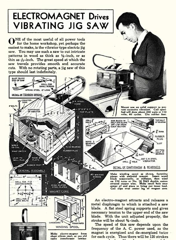
Drill and tap core for long, No. 12 screws.
