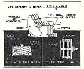
Variable condenser size formula is given above. Since spacing S and plate thickness are usually same, S may be calculated by measuring distance between outside plates of condenser.
