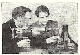
Operating drill made with Ford generator and set of parts.
