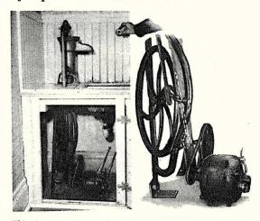
This home-made electrical contrivance for operating the kitchen pump fits under the sink and was built at small cost. Method of transmitting the power is shown at right above.
