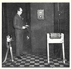
If a carrier of concealed firearms walks between magnets at jail door, a light and buzzer give warning signal to keeper.
