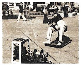
Line fastened to spool on motor shaft provides all the thrills of battling swordfish. Device keeps anglers in trim.
